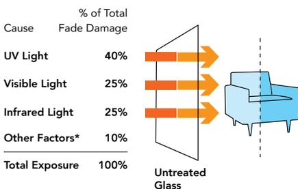
The sun's ultraviolet radiation, heat and light cause fading and deterioration of fabrics, carpets, furnishings, storefront displays and other interior items. All Solar Gard films reject up to 99% of harmful ultraviolet radiation, and varying amounts of heat and light. This helps dramatically reduce damage to your interiors and furnishings, keeping them in like-new condition longer.
