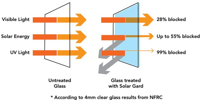
On clear 4mm (3/16") glass the sun's heat and light pour through. With Solar Gard LX 70 installed on your windows, over half of the sun's total solar energy is kept out, including over 99% of the ultraviolet light, while the visible light remains. Solar Gard LX 70 is like sunscreen for your environment.
