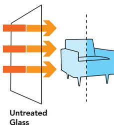
The sun's ultraviolet radiation, heat and light cause fading and deterioration of fabrics, carpets, furnishings, storefront displays and other interior items. All Solar Gard films reject up to 99% of harmful ultraviolet radiation, and varying amounts of heat and light. This helps dramatically reduce damage to your interiors and furnishings, keeping them in like-new condition longer.
